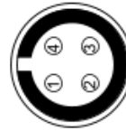
4 pins Binder 719 female connector pinout solder termination view
