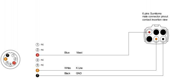
7 pins Binder 712 male connector pinout solder termination view
