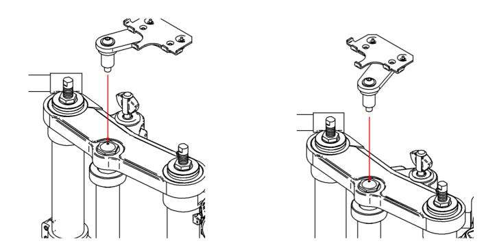
Tighten the central screw on the hinge so that this last grips.
