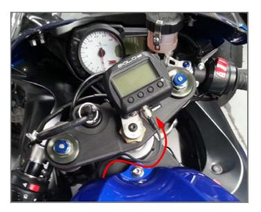
To connect SoloDL to male Binder connector of **V02569140** use the 7 pins female Binder connector placed bottom right of the logger as shown here below.
