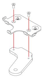
Screw the 8x45 pan head Allen screw in the toothed washer and screw the rubber loose piece under Suzuki adapter bracket.
