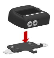
Fix it using the screws already inserted rear on Solo/SoloDL bracket.
