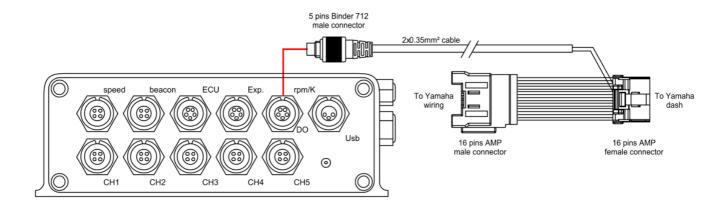
Connection between AiM EVO4 and Yamaha R1 2009-2013 (cable with JAE connectors) is shown here below.
