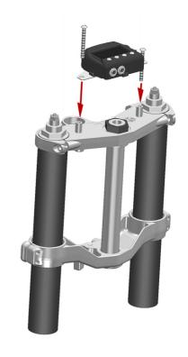
If your handlebars are not original lock the bolt with the nuts you find in the kit.
