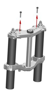
Insert in the screws housings the cylindrical distance pieces you find in the kit.
