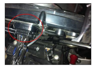
If you installed **EVO4**, take AiM cable – highlighted in the image – to it. If you installed a **SoloDL** make AiM cable pass around the bike stock dash.
