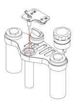
Screw the central screw on the hinge so that this last grips.
