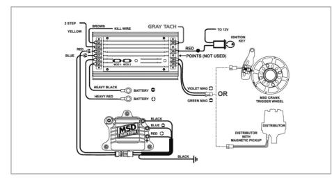
The output labelled "GRAY TACH" gives a 5-50V output that can be directly sampled by MX Strada series dash.
