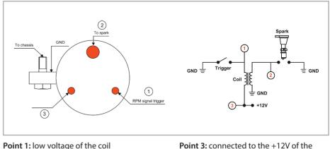
**Point 2:** connected to the spark plug
