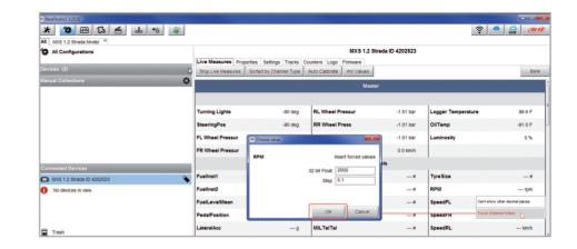
As shown in the image below, once the values have been forced they are shown right of the page hedged in red. With the two "+" and "-" lateral buttons it is possible to change the forced values.
