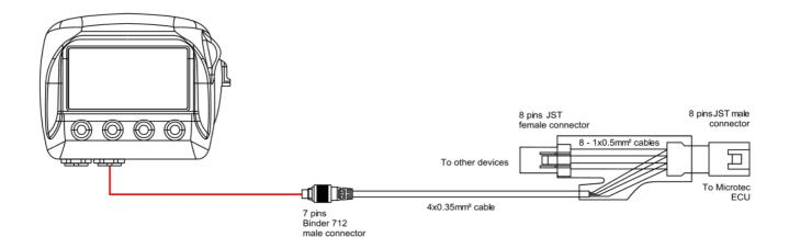
ECU connector has a cap on it. If the ECU is only connected to SoloDL remove the cap and place it on AiM kit female connector (labelled "to other devices" here above) and connect AiM kit male connector to the ECU female connector.
