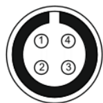
4 pins Binder 719 female connector pinout solder termination view
