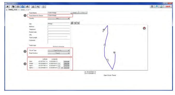
It is possible to change the start line position (move the cursor and set "Cursor Position") and to add split points in order to organize the track in different segments (**3**). This will be used in Data Analysis.
